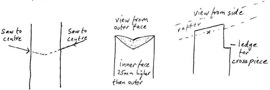
Note: point x is midpoint of upright where it supports rafter. You start cutting 25mm too high and cut down to this point. Try on a few spare off cuts first.
