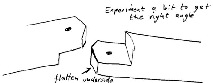
(diagram 3) Arrangement and joint detail for henge crosspieces.
