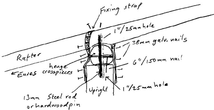
Note: Underside of rafter is shaped to take curve of crosspiece. Hole in rafter is bigger than rod, to allow play on erection and is at a slight angle. Fixing strap twists to allow nails into crosspieces.
