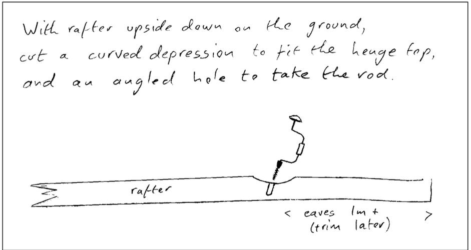
(diagram 5) Rafter detail for fixing at hinge crosspiece.
