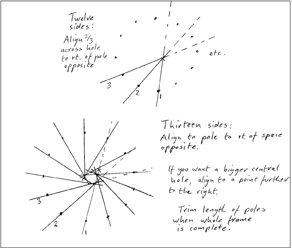
(diagram 4) Reciprocal roof frame rafter layout and placing sequence.
