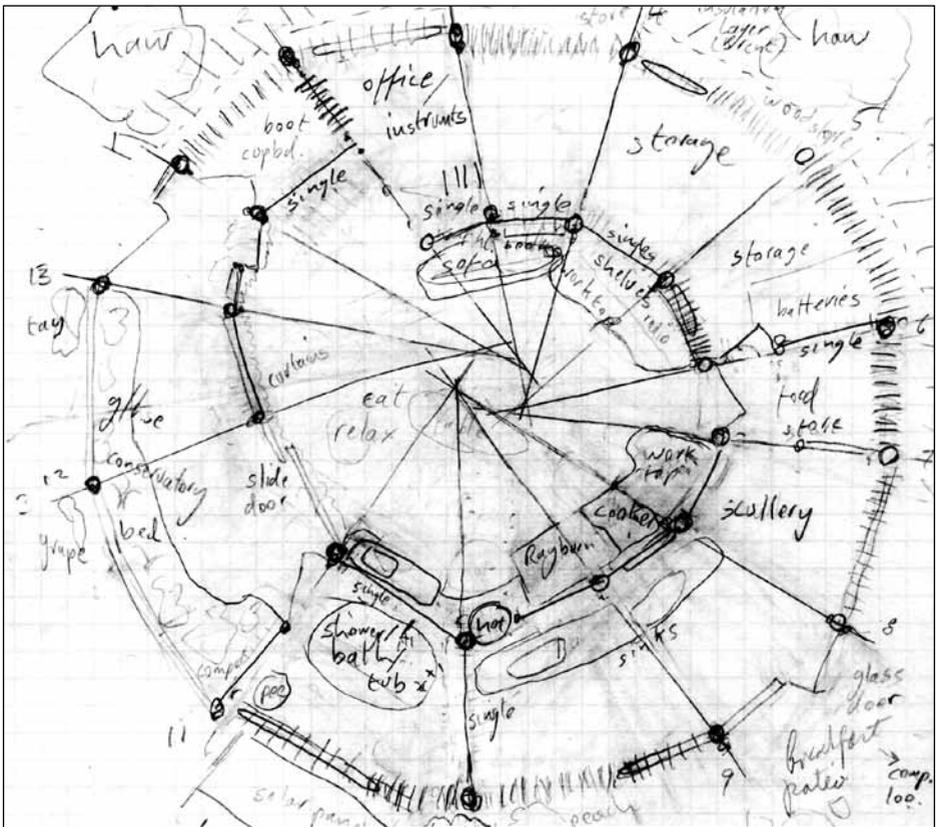
(diagram 1) This is about as detailed as any design got: post and beam structure, round, with reciprocal frame roof. Outer circle of uprights to go up first, then henge crosspieces, then roof. Cordwood in walls.
